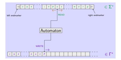
$$(Q, \Sigma, I, F, \delta) \xleftarrow{(A, \phi)} \text{production function: } \delta \to \Gamma \cup \{\epsilon\}$$
