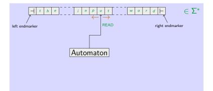
$$(Q, \Sigma, I, F, \delta) \xleftarrow[]{} (Q, \Sigma, I, F, \delta) \xleftarrow[]{} transition set: \subseteq Q \times \overline{\Sigma} \times \{-1, 0, +1\} \times Q$$
